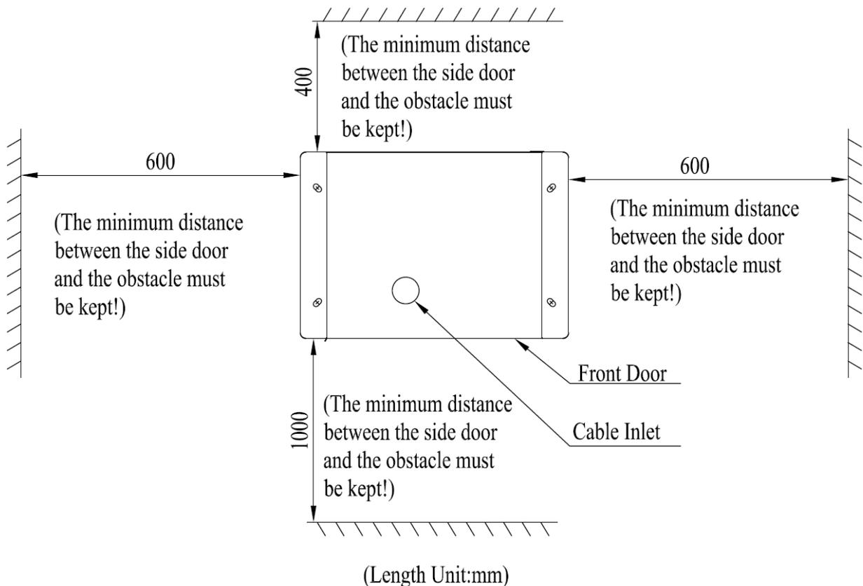
**Figure 3.2-A Requirements for charger placement**
