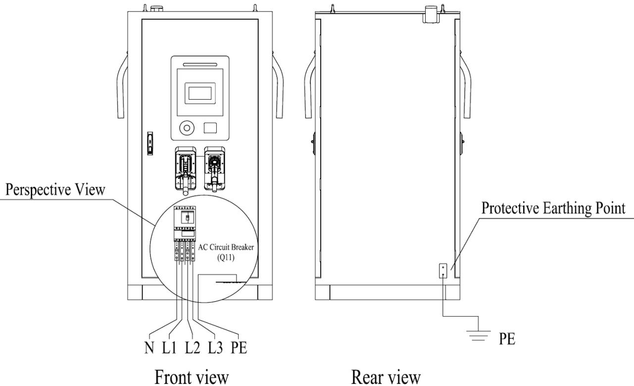
**Figure 3.4-A Internal wiring diagram of charger**
