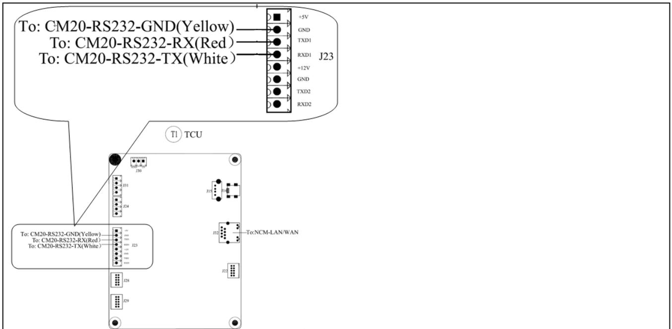
**Note:** the following cables of the TCU(T1) needs to be connected:
