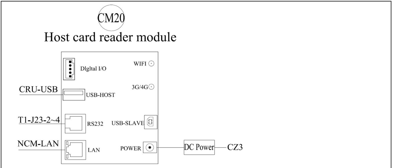
**Note:** the following cables of the host card reader module (CM20) needs to be connected
